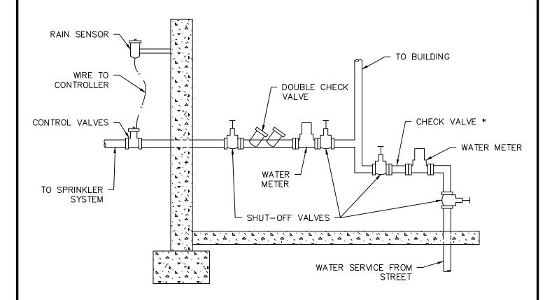
\* COMMERCIAL BUILDINGS ARE REQUIRED TO HAVE EITHER A DOUBLE CHECK VALVE (WATTS 007 OR SIMILAR), OR A REDUCED PRESSURE ZONE ASSEMBLY (WATTS 009 OR SIMILAR), DEPENDING ON BUILDING USE.
